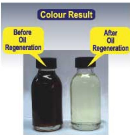
**Regeneration of transformer oil in the transformer tank is technically superior and more cost effective than the alternative procedure known as draining, flushing and refilling, as all the acidic oil is removed from the insulation material which will contaminate replaced oil.**
